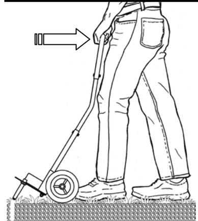
*To avoid excessive wear, do not use the Step 'N Tilt™ lawn aerator when the ground is dry.*
