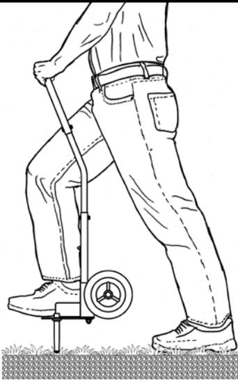
2: Step on the platform directly above the aerator tine (do not push down on the handle with your hands). The deflectors will prevent the soil cores from dropping onto the stepping platform.
